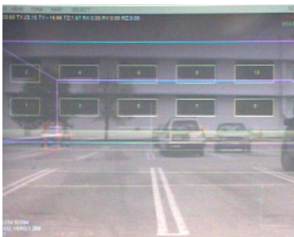
Figure 1: Image captured from a see-through augmented reality system. Various computer-generated annotations are overlaid directly on objects in the user’s environment.
