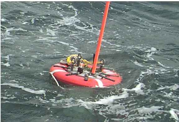
Fig. 10. In Seawebs '98, '99, and 2000, a Racom buoy provides a very reliable line-of-sight packet-radio link to Seaweb servers at the ashore command center and on the work boat. The radio link is a 900-MHz spread-spectrum technology commercially known as Freewave. In Seawebs '99 and 2000, additional gateway nodes using cellular modems linked via Bell Atlantic and the Internet provide even greater flexibility and provide access by Seaweb servers at various locales across the country.
